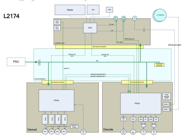
As shown in the block diagram above, the Demodulator board generates an ASI stream from the RF inputs and/or the external ASI, then passes this to the Decoder board to generate the Video and Audio outputs. In addition, the Decoder extracts embedded (or 'wayside') RS232 data if it is present in the transmission, as well as return data from a VISLINK Camera Control System. There are 2 ASI connections between the boards to allow extra flexibility in how the unit is configured (see later).
