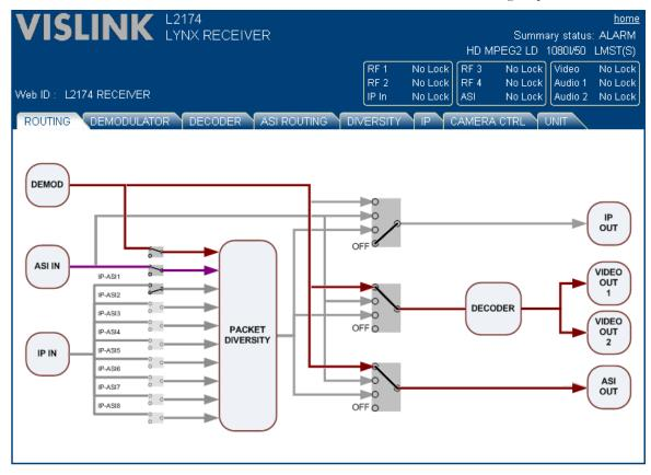
If a box is 'greyed' then that indicates that the feature is not licensed. If a box changes colour when the mouse 'hovers' over it, then clicking will take the operator to the relevant page to configure that function. The switches change state when clicked, and will cycle through the available options. V0015 code will only perform Packet Diversity between the ASI and RF ports, therefore the input switches are fixed as shown.
